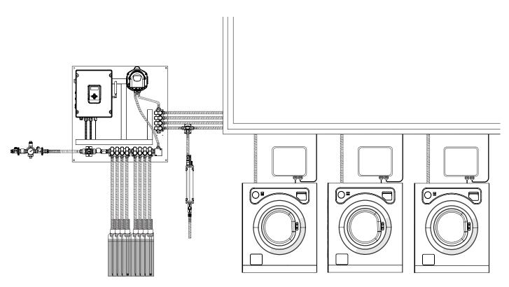
This image reproduces the 'Standard' setup of a Multiplex unit with one channel (your setup will vary based on model), understanding "Channel" as a group of products that are injected into the same manifold and directed to a distributor (washing machines) or an injection (tunnel).
