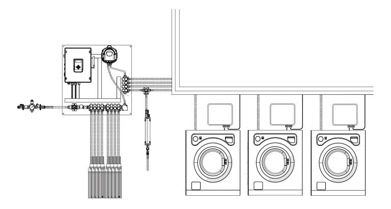
This image reproduces the 'Standard' setup of a Multiplex unit with one channel (your setup will vary based on model), understanding "Channel" as a group of products that are injected into the same manifold and directed to a distributor (washing machines) or an injection (tunnel).
