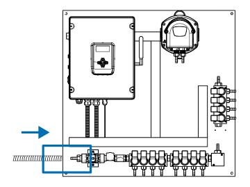
Connect the water supply to the water inlet connection seen on the unit here.
