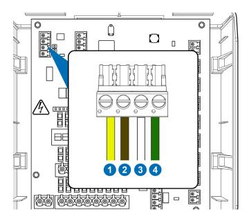
To connect the external communication box to the unit, connect terminal X2 on the main machine to terminal X1 on the communication box.
