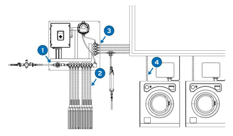
To connect equipment, distributor and washers, use 10x16 braided PVC pipe and stainless steel clamps.
