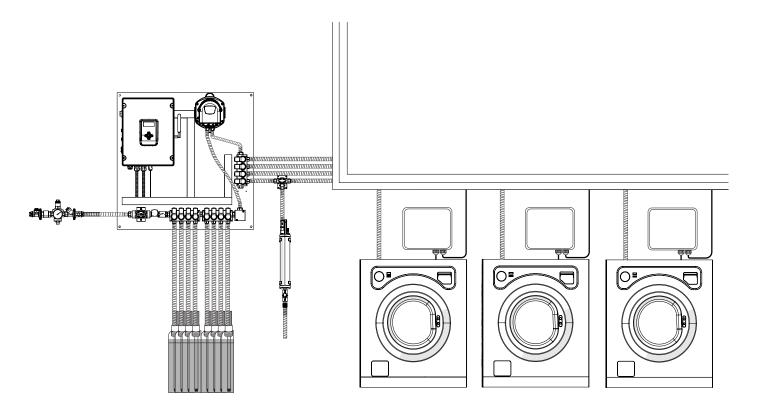
This image reproduces the 'Standard' setup of a Multiplex unit with one channel (your setup will vary based on model), understanding "Channel" as a group of products that are injected into the same manifold and directed to a distributor (washing machines) or an injection (tunnel).
