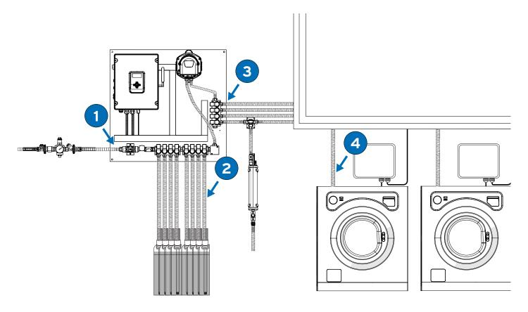
To connect equipment, distributor and washers, use 10x16 braided PVC pipe and stainless steel clamps.
