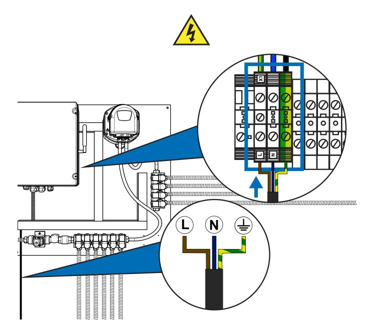
For the power supply of the equipment you must use 3x1′5mm2 cable. Insert the cable through the channel located at the bottom left and use one of the cable glands to insert it safely inside the control cabinet. Connect to the terminals identified with X1 found on the lower left of the connections.
