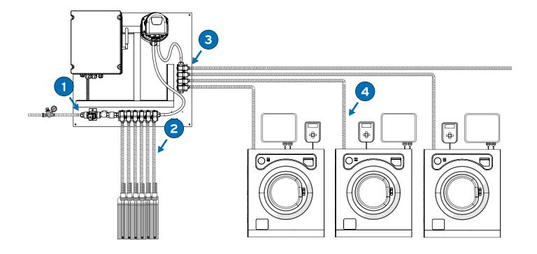
To connect equipment, distributor and washers, use 10x16 braided PVC pipe and stainless steel clamps.
