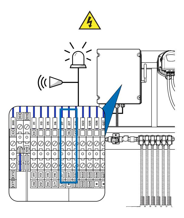
To connect an external alarm or warning light to the system, utilize slot X6 as depicted above.
