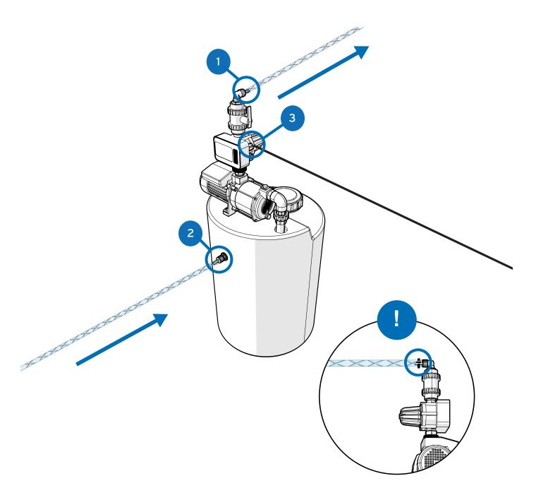
Please note that the unit requires a flow rate of min 2/I per min - max 10/I per min and a dynamic pressure range of 1.5 bar (min) - to 3 bar (max). A booster tank is recommended whenever a consistent supply is not available.
