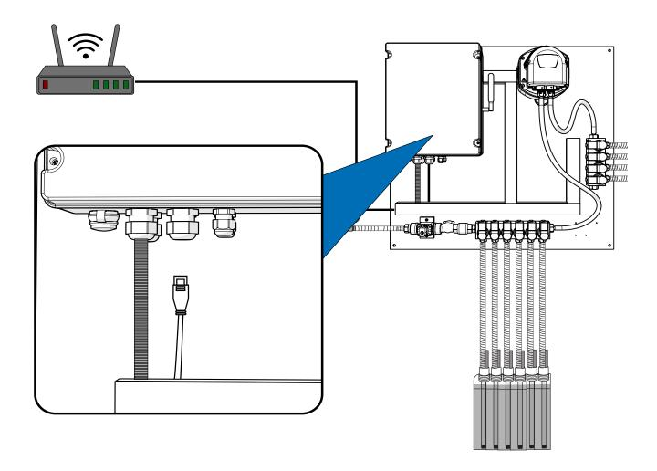
To connect your unit to the internet, simply plug an Ethernet cable into any router through the connector located on the bottom of the main box.
