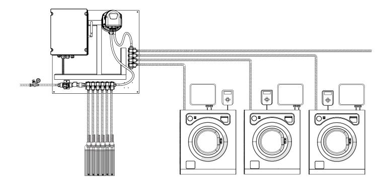
This image reproduces the 'Standard' setup of a Multiplex unit with one channel, understanding "Channel" as a group of products that are injected into the same manifold and directed to a distributor (washing machines) or an injection (tunnel).
