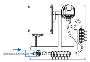
Connect the water supply to the water inlet connection seen on the unit here.
