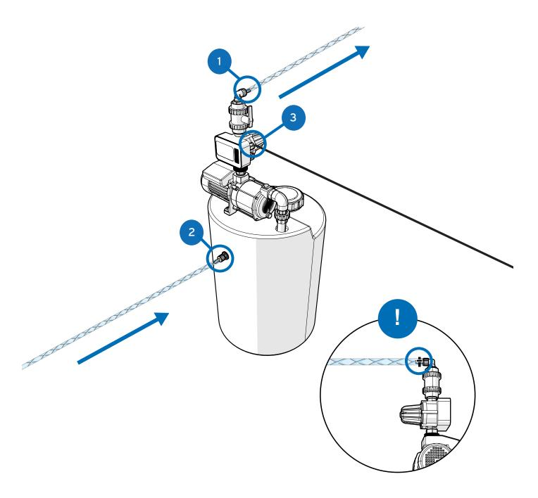
Please note that the unit requires a flow rate of min 2/I per min - max 10/I per min and a dynamic pressure range of 1.5 bar (min) - to 3 bar (max). A booster tank is recommended whenever a consistent supply is not available.
