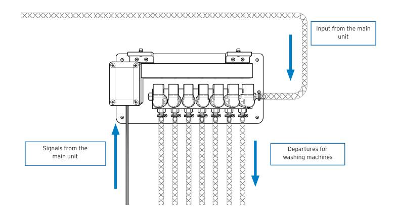
28 ELECTRICAL WIRING SUCTION RODS
