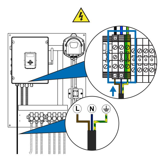
For the power supply of the equipment you must use 3x1'5mm2 cable. Insert the cable through the channel located at the bottom left and use one of the cable glands to insert it safely inside the control cabinet. Connect to the terminals identified with X1 found on the lower left of the connections.
