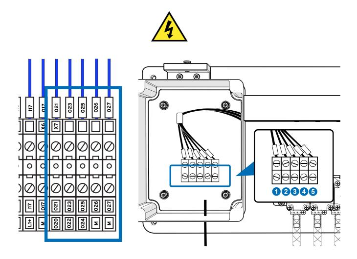
Use a **7x18 AWG** cable for the connection between the control cabinet and the distributor. Connect the distributor to terminal block **X7**. Each terminal connection corresponds to the outlets numbered from left to right, with the number dependent on the order. Below is the wiring diagram for the main unit.
