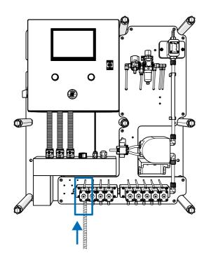
Connect the water supply to the leftmost pneumatic valve on the central panel of the unit.
