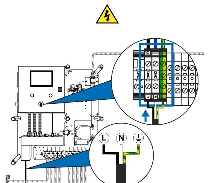
For the power supply of the equipment you must use **3x16 AWG cable**. Insert the cable through the channel located at the bottom left and use one of the cable glands to insert it safely inside the control cabinet. Connect to the terminals identified with **X1** found on the lower left of the connections.
