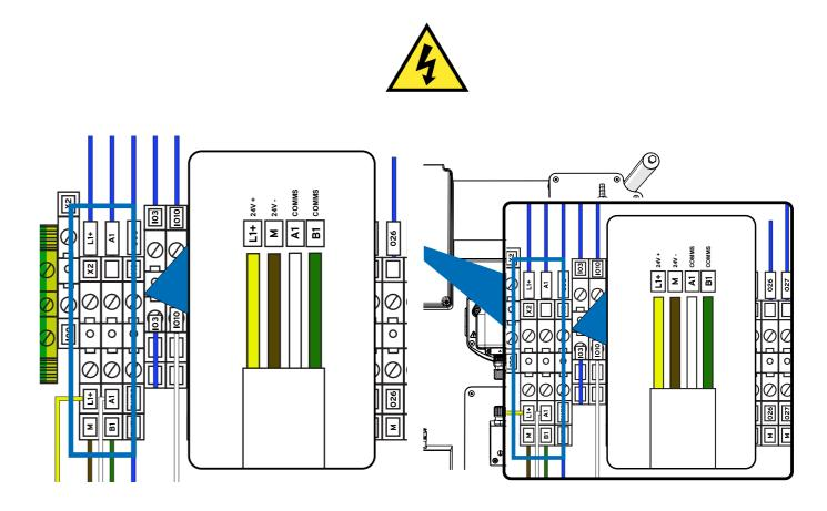
To connect the expanision channel to the unit, connect X2 on the main machine to X1 on the expansion channel.
