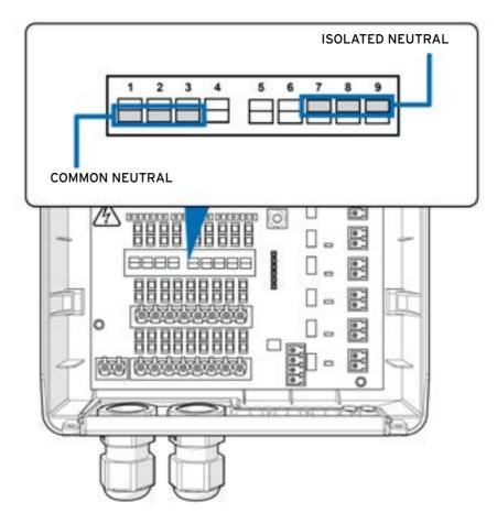
COMMS WIRING SIGNAL BOX CONNECTING YOUR EXTERNAL DISTRIBUTOR
