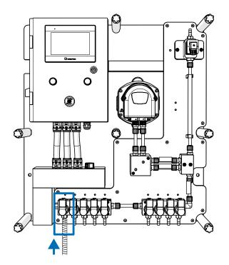
Connect the water supply to the leftmost solenoid valve on the central panel of the unit.
