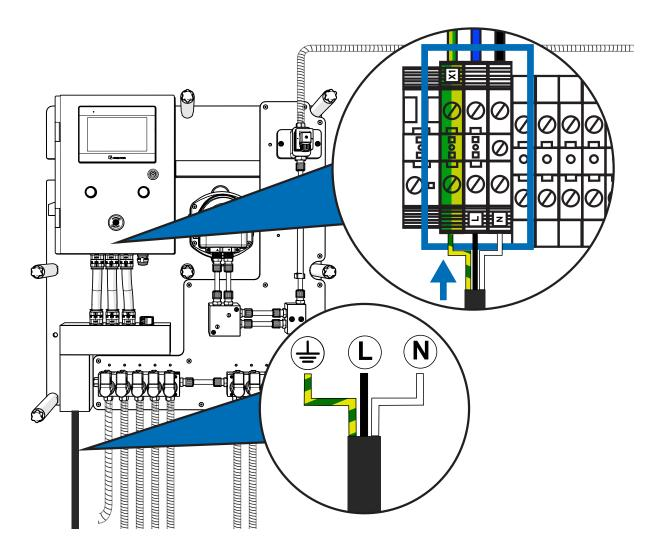
For the power supply of the equipment you must use **3x16 AWG cable**. Insert the cable through the channel located at the bottom left and use one of the cable glands to insert it safely inside the control cabinet. Connect to the terminals identified with **X1** found on the lower left of the connections.
