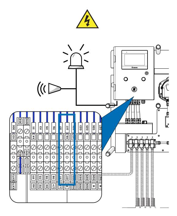
To connect an external alarm or warning light to the system, utilize slot X6 as depicted above.
