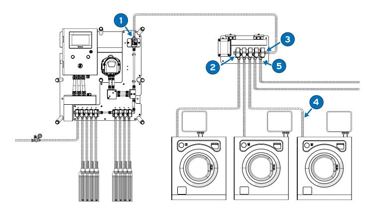
To connect equipment, distributor and washers, use 3/8" ID x 1/2" OD mesh PVC pipe and stainless steel clamps.
