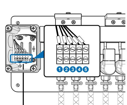
Use a 7x1mm^2 cable for the connection between the control cab inlet and the distributor. Connect the distributor to terminal block X7. Each terminal connection corresponds to the outlets numbered from left to right, with the number dependent on the order. Below is the wiring diagram for the main unit.
