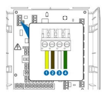
To connect the external communication box to the unit, connect terminal X2 on the main machine to terminal X1 on the communication box.
