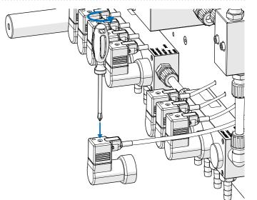
REPLACING A VALVE ON YOUR MULTIPLEX SYSTEM MAINTENANCE
