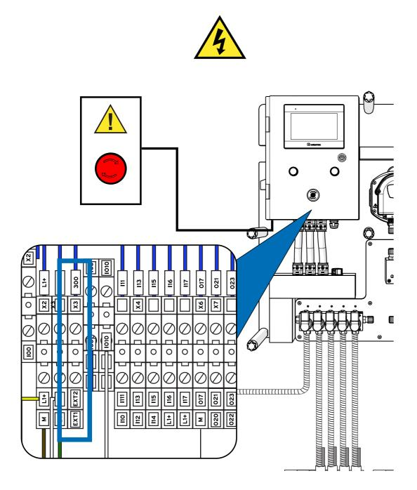
To connect an emergency stop button to your unit, you can use the EXT1 and EXT2 connectors slot shown above in series.
