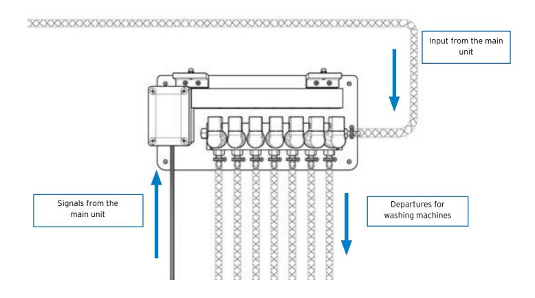
28 SIGNAL WIRING EXTERNAL DISTRIBUTOR ELECTRICAL WIRING SUCTION RODS
