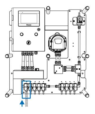
Connect the water supply to the leftmost solenoid valve on the central panel of the unit.
